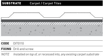
NUTE Installed on top of, or recessed into, any existing carpet substrate that cannot be removed including steel access floors. Custom plate sizes available.
